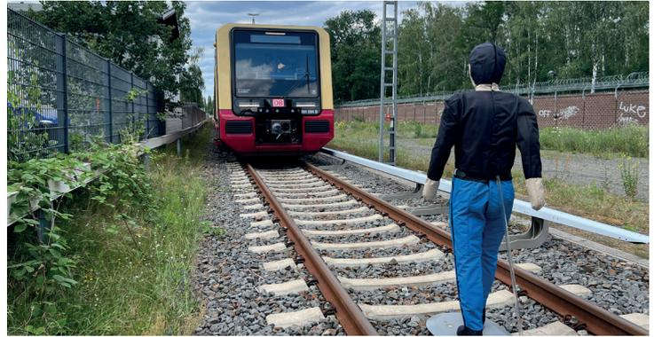
BerDiBa project – test of automatic obstacle detection
