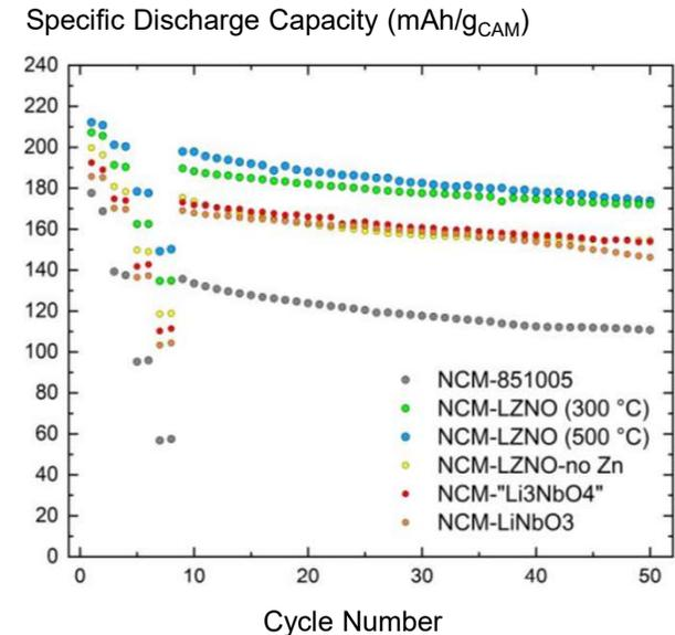
Despite high (>10 nm) thickness, coating has sufficient ionic conductivity
