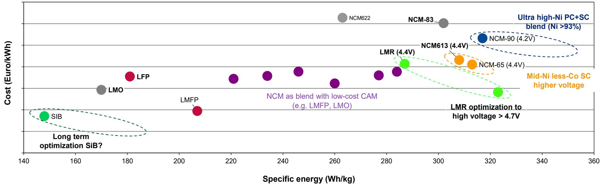
Parameter field to optimize cost vs performance on CAM material level
