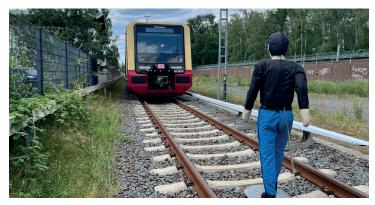
BerDiBa project – test of automatic obstacle detection
