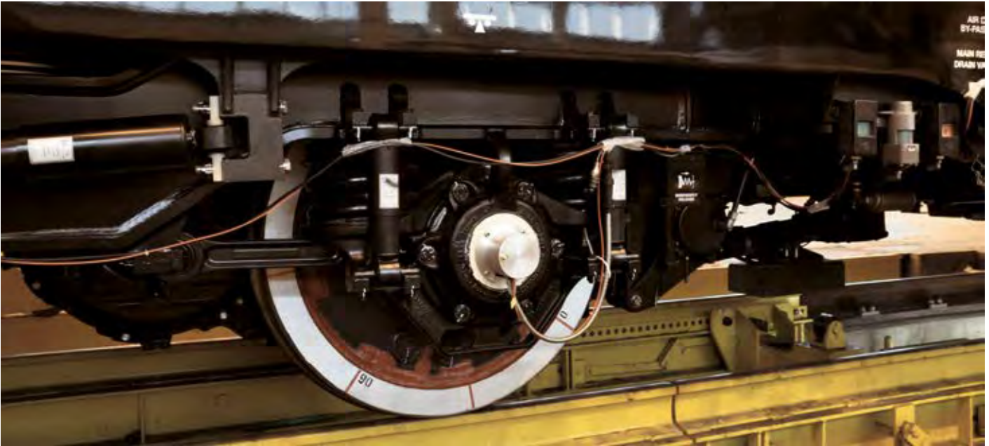
Locomotive ALP-45DP with a PROSE measuring wheelset ready for use at the New Jersey Transit Meadows Maintenance Center
