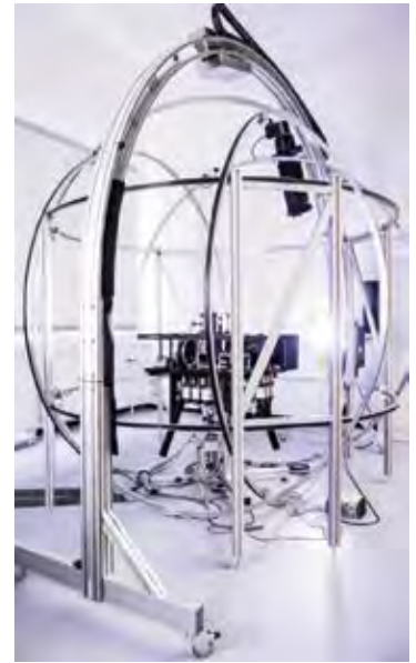
Attitude Control System - test stand for small satellites
